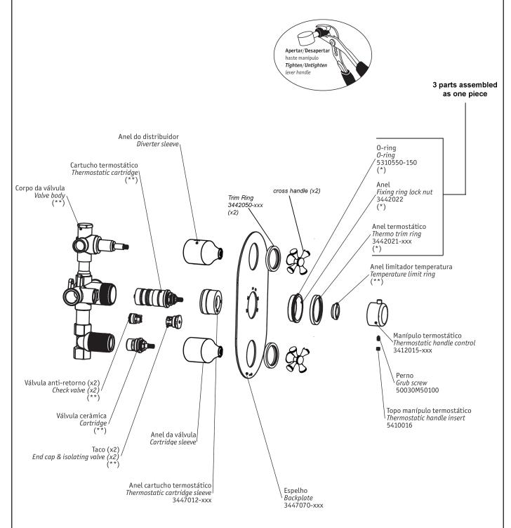
Notes: 1) The red dot on the temperature limit ring must be aligned with the number 38 on the handle, ie @ 12 o'clock
