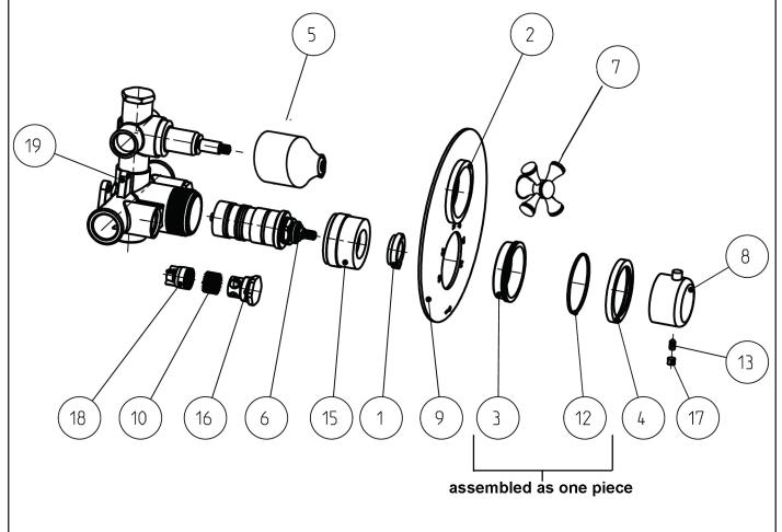
Notes: 1) The red dot on the *temperature limit ring* must be aligned with the number 38 on the handle, ie @ 12 o'clock 2) Part Numbers 3, and 12 are Pre-assembled at factory and come as one piece
