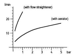
IF THE PRESSURE IS HIGHER THAN 1 bar REMOVE FLOW STRAIGHTENER AND REPLACE WITH AERATOR PROVIDED
