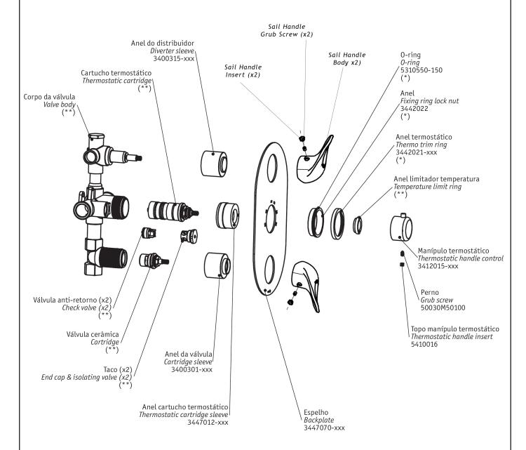
Notes: 1) The red dot on the temperature limit ring must be aligned with the number 38 on the handle, ie @ 12 o'clock
