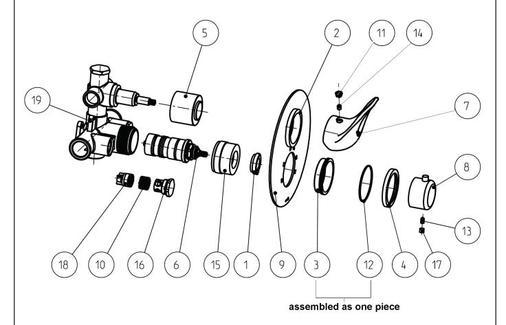
1) The red dot on the *temperature limit ring* must be aligned with the number 38 on the handle, ie @ 12 o'clock 2) Part Numbers 3, and 12, are Pre-assembled at factory and come as one piece
