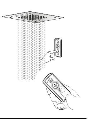
**Note:** a remote control can be associated to several showerheads to control them at the same time. It is not possible, on the contrary, to control a single showerhead with several remote controls.
